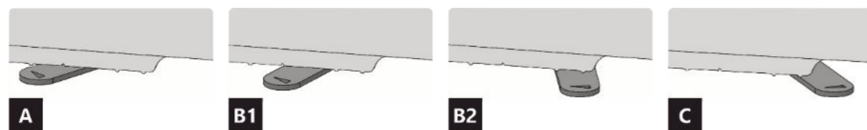
Fig. 9 Air intake controller – type 5
