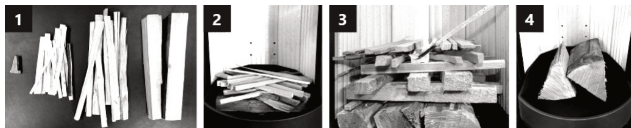
Fig. 4 Placements of wood in the chamber
